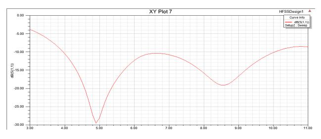
FIGURE 7-THE RETURN LOSS CHARACTERISTICS (S11 PARAMETERS) OF THE ANTENNA WITH THE DESIGN 2
