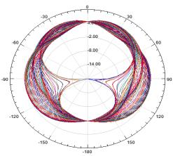
FIGURE 5-RADIATION PATTERN AT ALL  $\phi$  AND AT FREQUENCY=6 GHz
