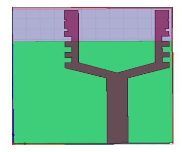
FIGURE 6- THE PROPOSED ANTENNA IN HFSS SOFTWARE.(TOP VIEW) WITH SLOTS OF DESIGN 2
