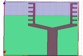
FIGURE 2- THE PROPOSED ANTENNA IN HFSS SOFTWARE.(TOP VIEW) WITH SLOTS EQUALLY CUT OF DIMENSIONS 1.5mm\*1.5mm
