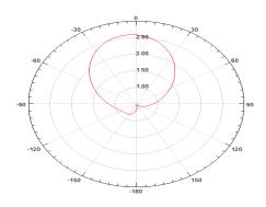
FIGURE 4-RADIATION PATTERN AT φ=0 AND AT FREQUENCY=6 GHz
