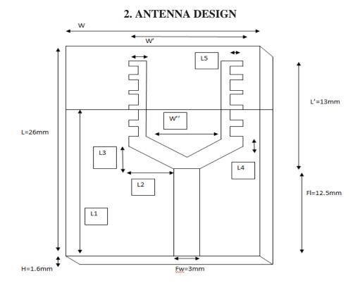
L1=19.5mm L2=7mm L3=2mm L4=2mm L5=1.5mm W''=11mm W'=15mm W=23mm L1 is for ground plain at the bottom of the substrate
